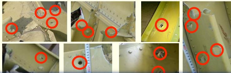
**DAMAGES TO SUPERSTRUCTURE (MAIN FRAMES) ARE LOCATED MUCH FURTHER AWAY FROM DAMAGES TO OUTER SKIN**
