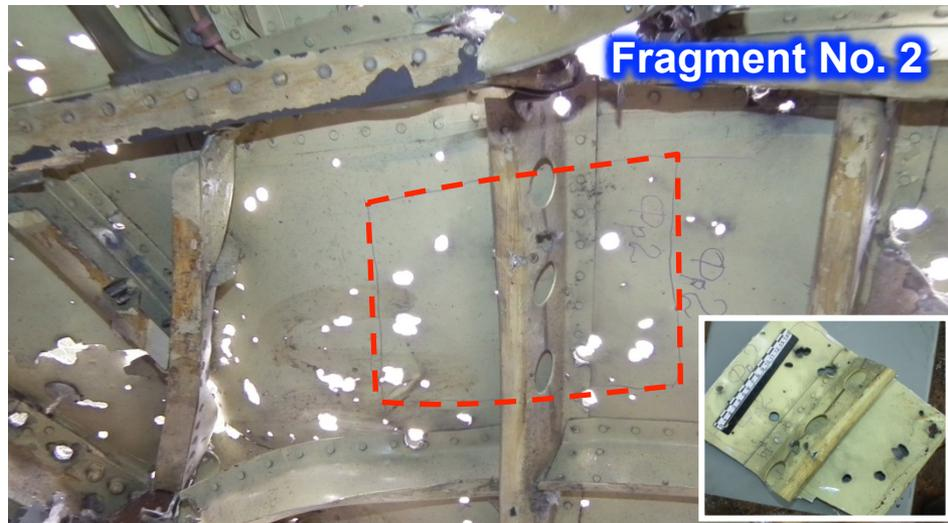
Port side structural element in the area of the PIC's side window
