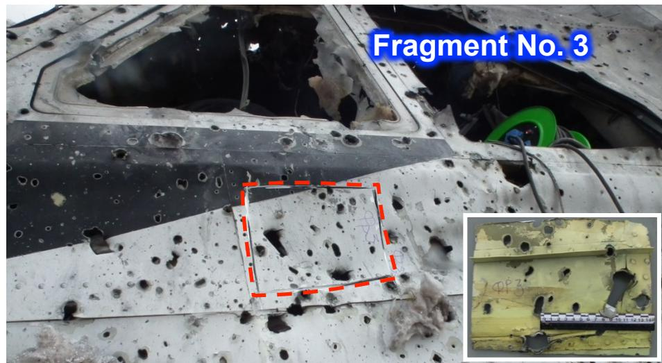
Roof structural member above the PIC's seat
