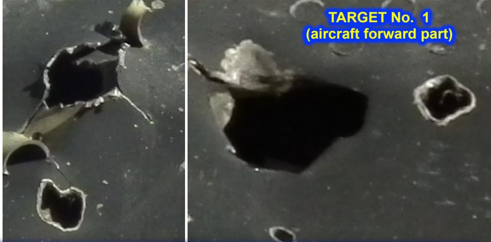
**DAMAGES TO THE ENGINE ARE DELINEATED BY COMBINATION OF ARMED SUB-MUNITIONS AND FRAGMENTS OF WARHEAD BODY BAY IMPACTING IN MAIN FIELD OF DEBRIS**
