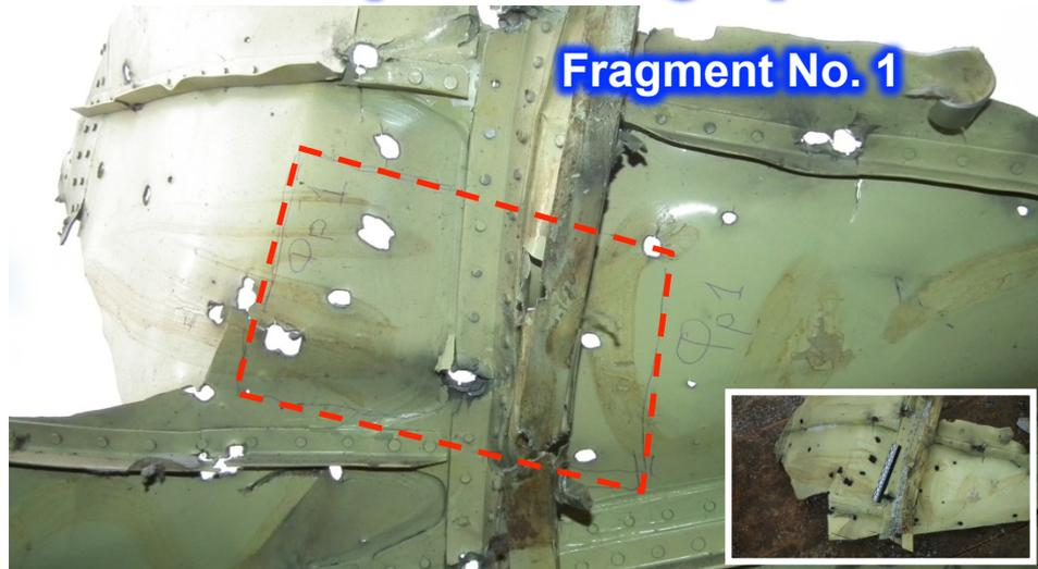
Roof structural member (complete with the stringer) of above the PIC's seat
