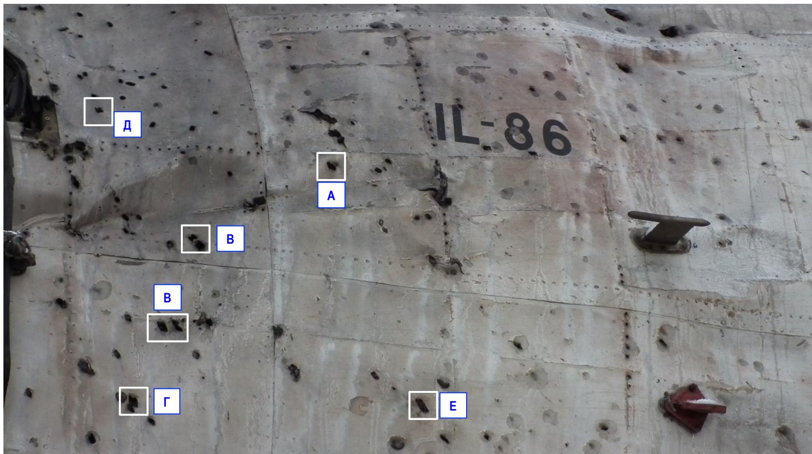
**Typical holes from I-BEAM submunitions (13x13x8,2 mm)**
