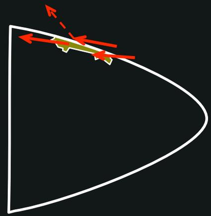
**1. The break-up of the structural members (main frames) in the area of the left-hand side cockpit canopy could be caused only by a submunition moving along the aircraft body.**
