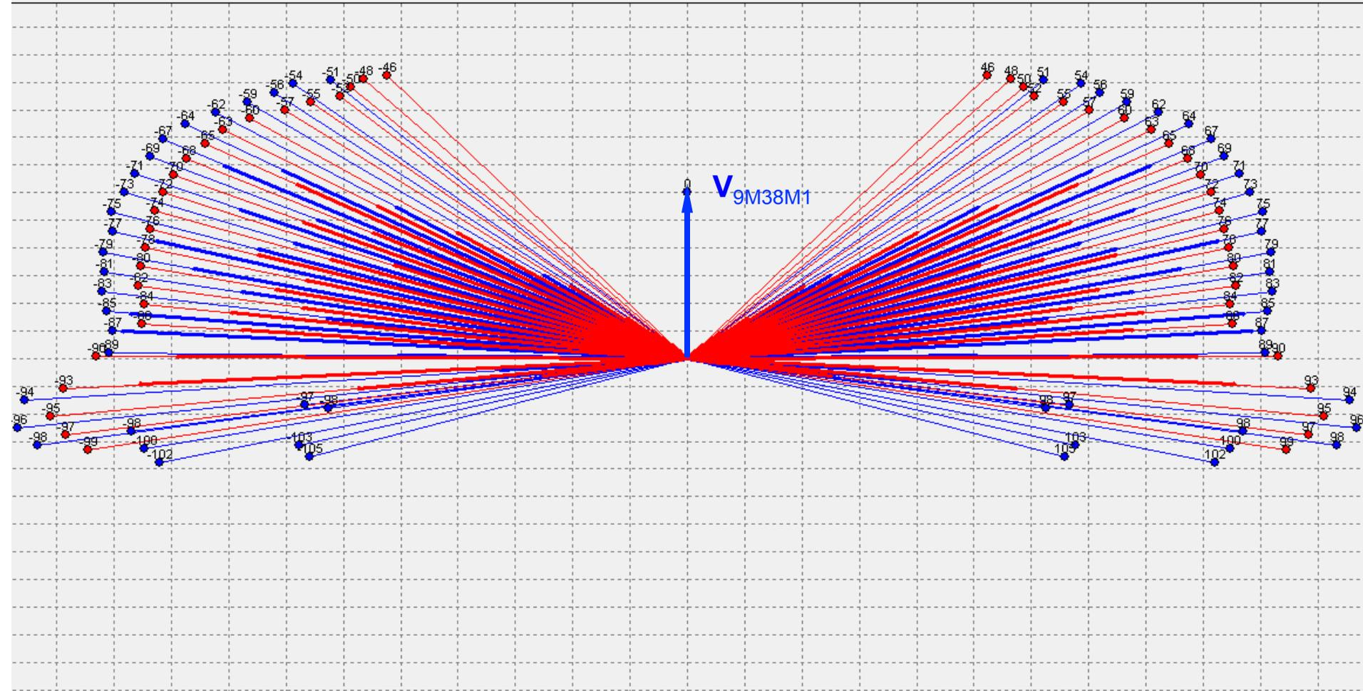
→  $V_{9M38M1} = 600$  m/s    →  $V_{B777} = 0$  m/s
