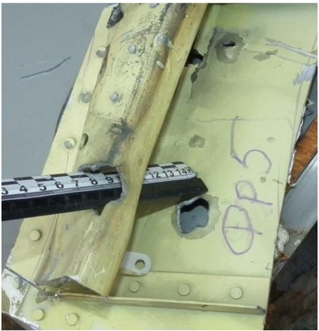
Port side structural element behind the PIC's seat
