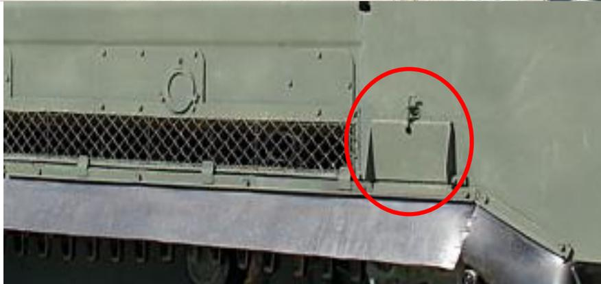
*Photograph of SPML Buk of 9A310M1-2 modification with folding platform*
